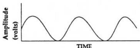
The sound's amplitude, or relative loudness, is shown by the height of the waveform. Its pitch is represented by frequency, or number of peaks per second. Frequency is expressed in Hertz: one cycle per second is a frequency of one Hertz. The lower the frequency, the lower the pitch of the sound.
