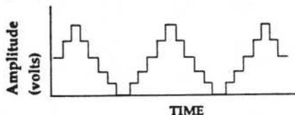
Once Digital Ears has converted the analog signal to a discrete binary number, the value is transmitted to the NeXT's DSP chip. Software that accesses the DSP can then process the data for analysis, display, or storage.
